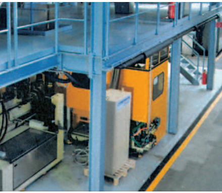
Preform machine in pilot plant
